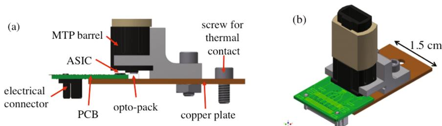
**Fig. 1.** (a) Schematic drawing of an opto-board together with a MTP barrel fastened to the opto-board for the insertion of a fiber ribbon terminated with MTP connector to receive the optical signal from the VCSEL array. (b) A three-dimensional rendition of the setup.
