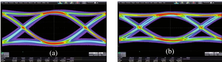
**Fig. 3.** Optical eye diagram of a VCSEL operating at 5 Gb/s before (a) and after (b) irradiation.
