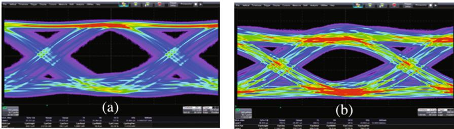
**Fig. 2.** Optical eye diagram of a VCSEL operating at 10 Gb/s before (a) and after (b) irradiation.
