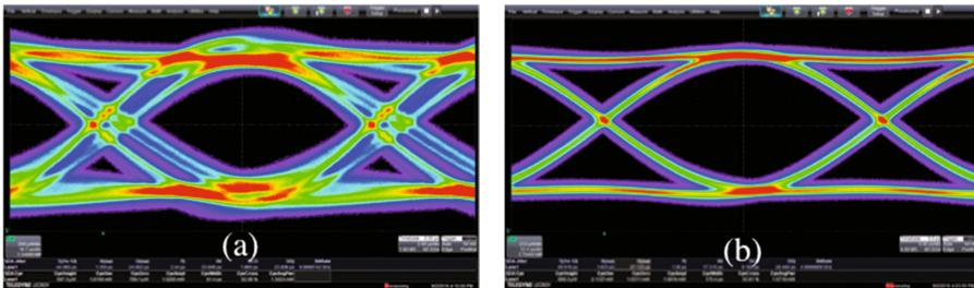
**Fig. 4.** Optical eye diagram of a VCSEL in the second prototype ASIC operating at 10 (a) and 5 (b) Gb/s.
