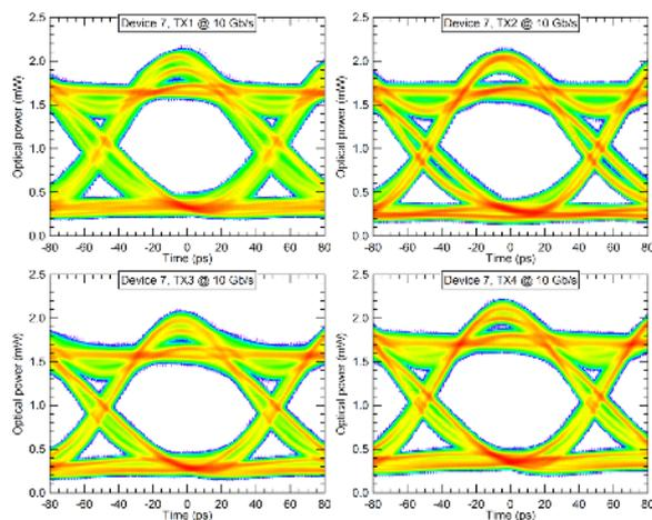
**Fig. 6.** Optical eye diagram for a 4-channel VCSEL array in a VTRx.
