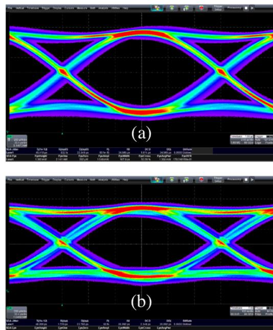
**Fig. 2.** Optical eye diagram of a VCSEL operating at 5 Gb/s before (a) and after (b) irradiation.
