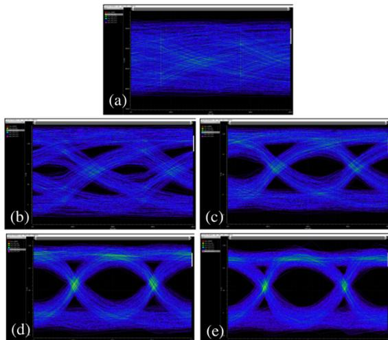
**Fig. 4.** Eye diagram of the electrical signal at the end of 5.5 m of skinny cable (a) and output at each of the four taps (b-e).
