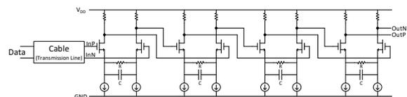
**Fig. 3.** 4-tap Continuous Linear Time Equalization (CTLE) circuit to equalize the frequency spectrum of a signal after emerging from a 5.5 m of skinny cable.
