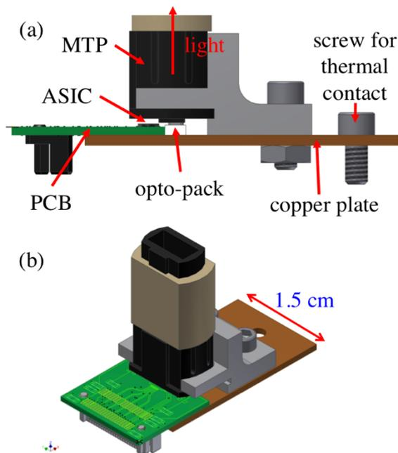
**Fig. 1.** (a) Schematic drawing of an opto-board together with a MTP barrel fastened to the opto-board for the insertion of a fiber ribbon terminated with MTP connector to receive the optical signal from the VCSEL array. (b) A three-dimensional rendition of the setup.
