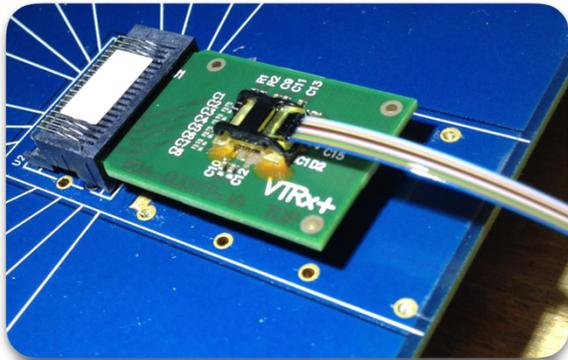
Fig. 8. A VTRx with an optical package attached to a fiber ribbon.
