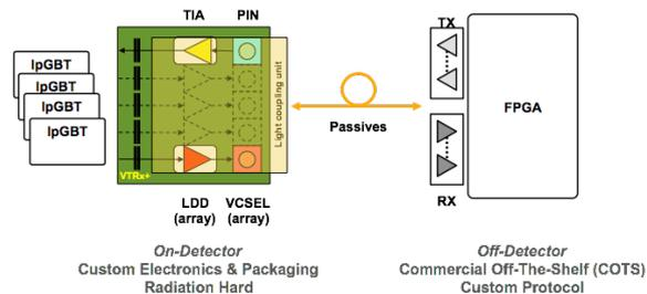
**Fig. 5.** Schematic of the data transmission system of the Versatile Link project.
