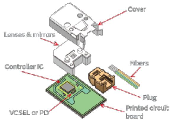
Fig. 9. A compact optical package by FOCl.
