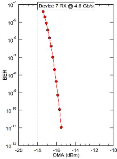
Fig. 7. Bit error rate of a receiver in a VTRx as a function of the optical modulation amplitude (OMA).
