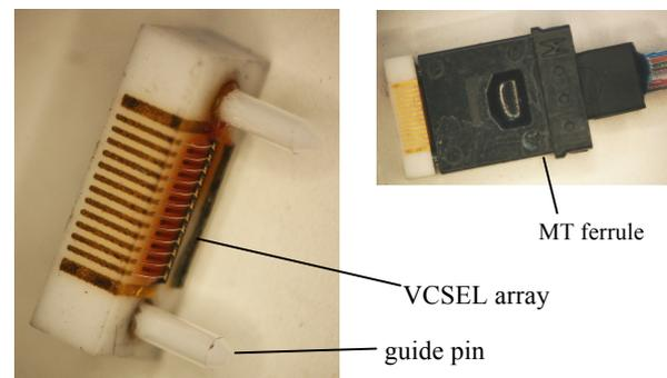
Figure 4: A fabricated opto-pack based on BeO.
