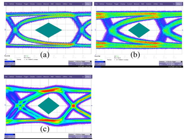
Figure 1: Eye diagrams of (a) 640 Mb/s signal after 1.4 m of cable, (b) 320 Mb/s signal after 3 m of cable, (c) pre-emphasized 320 Mb/s signal after 4 m of cable.
