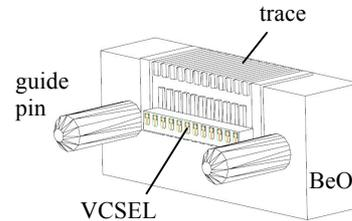
Figure 3: An optical package based on BeO.
