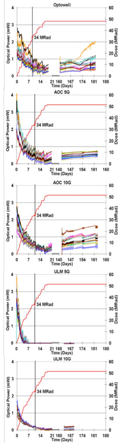
Figure 2: Optical power as a function of time (dosage) for various VCSEL arrays that transmitted data to the control room. The power decreased during the irradiation but increased during the annealing as expected. The arrays were returned to The Ohio State University after  $\sim 140$  days for an extended annealing and there are some recovery of the power except the ULM 5 Gb/s arrays.
