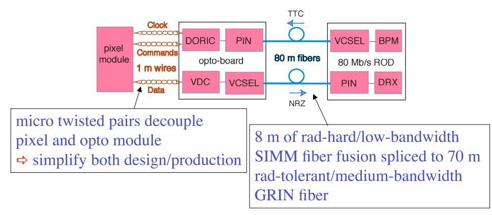
Plan: upgrade based on current pixel link architecture
