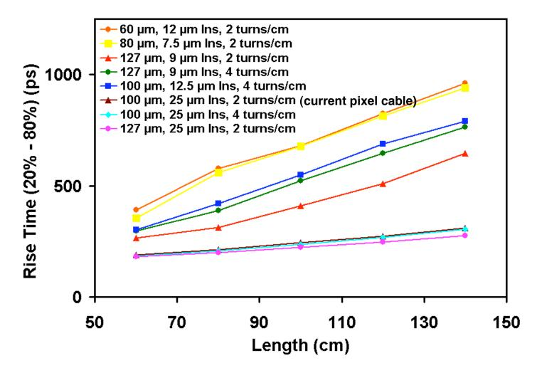
• current pixel cable with thick insulation is quite optimum! K.K. Gan B Layer Workshop 12
