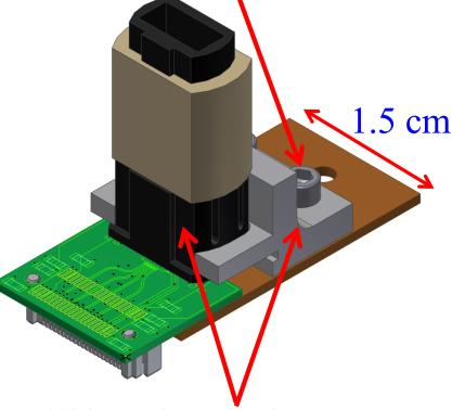
Will be fabricated as one piece with mold injection to reduce the width
