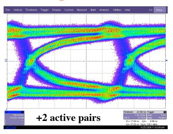
• LVDS signal after 6 m of wires looks adequate
