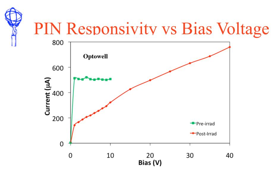
can fully recover pre-irradiation responsivity with high bias voltage
