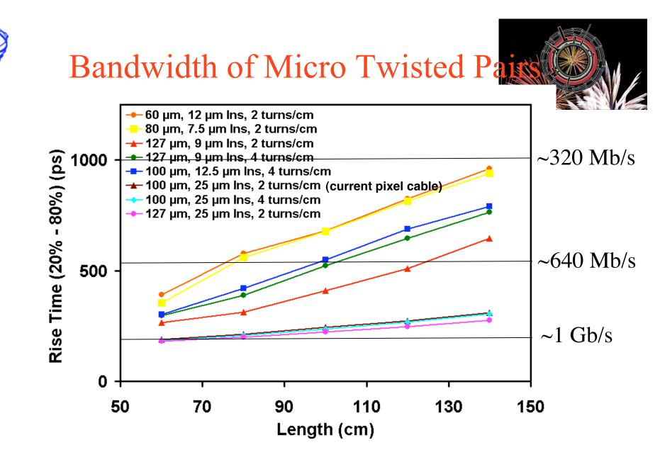
• current pixel cable with thick insulation is quite optimum! K.K. Gan ATLAS Tracker Upgrade Workshop 4
