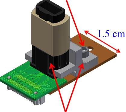
Could be fabricated as one piece with mold injection
