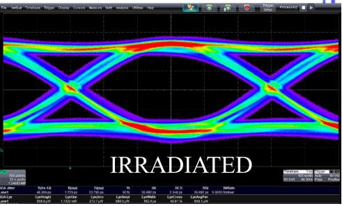
• performance of the array driver/VCSEL combination at 5 Gb/s is acceptable after irradiation
