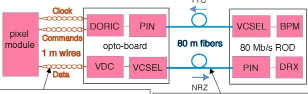
micro twisted pairs decouple pixel and opto module
