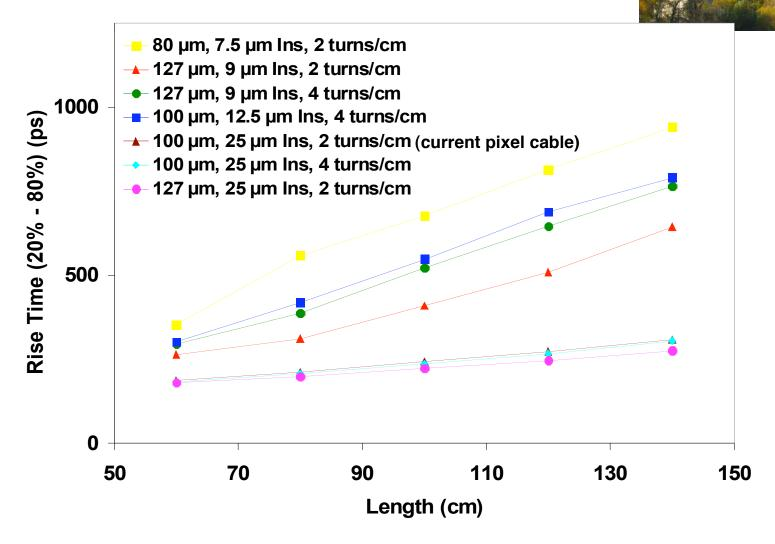
• current pixel cable with thick insulation is quite optimum!
