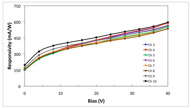
• can fully recover pre-irradiation responsivity with high bias voltage
