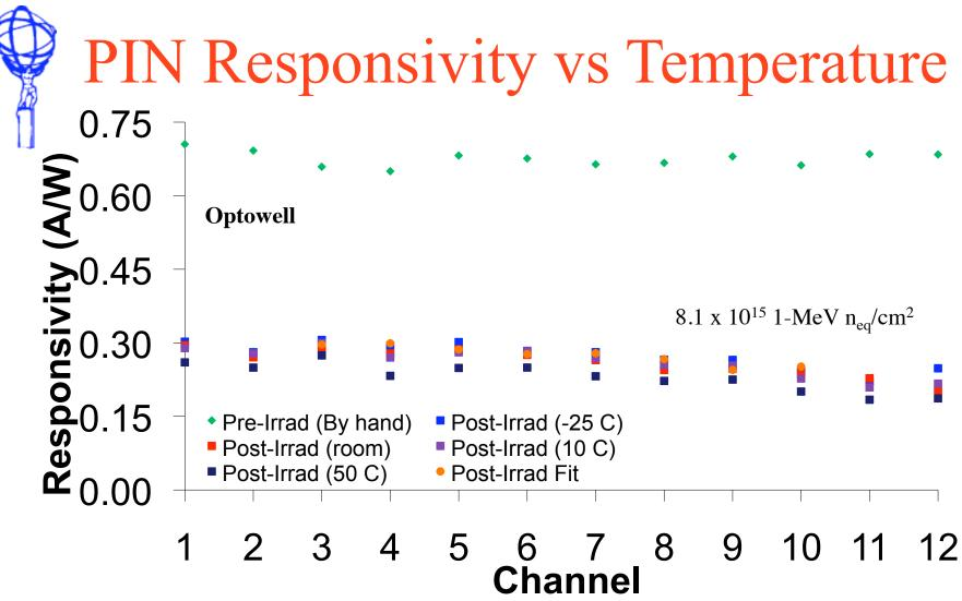
Responsivity is slightly higher at lower temperature
