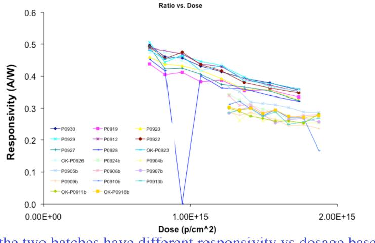
• the two batches have different responsivity vs dosage based on naive assumption of linear proton flux vs channel number
