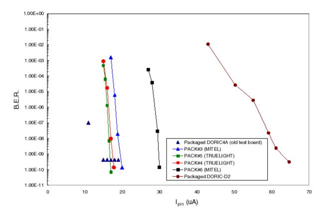
opto-link can run with no bit error at low PIN current
