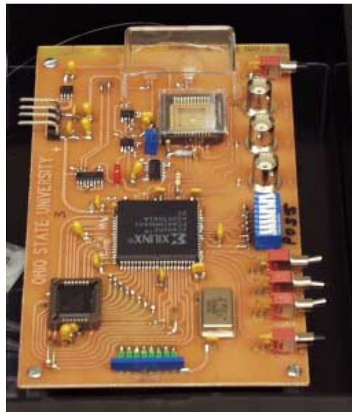
Bit error test board in control room ( 4 boards)
