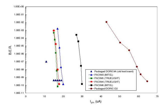
• opto-packs can run with low PIN current
