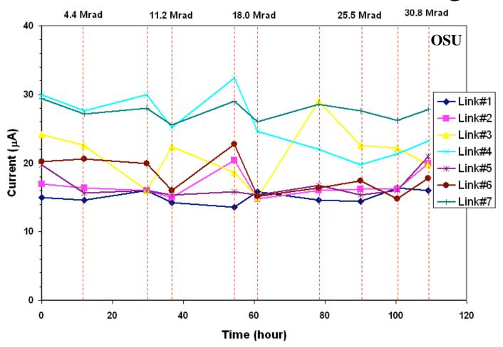
• PIN current thresholds for no bit errors remain constant
