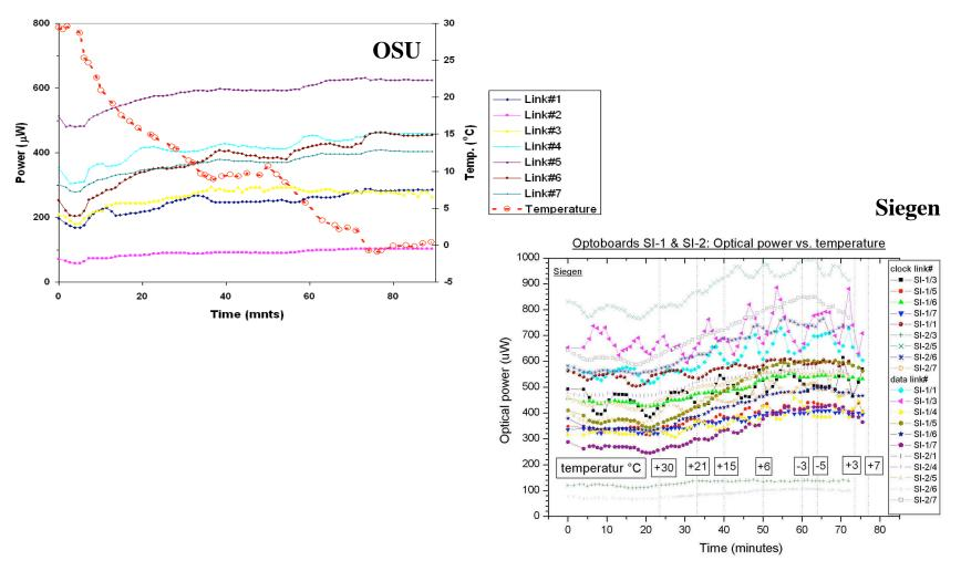
• cooling opto-board increases optical power by 10-30%
