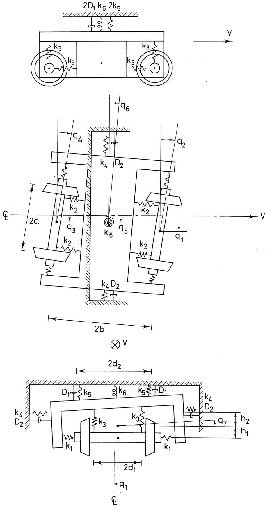
Fig. 2. Conventional bogie model.
