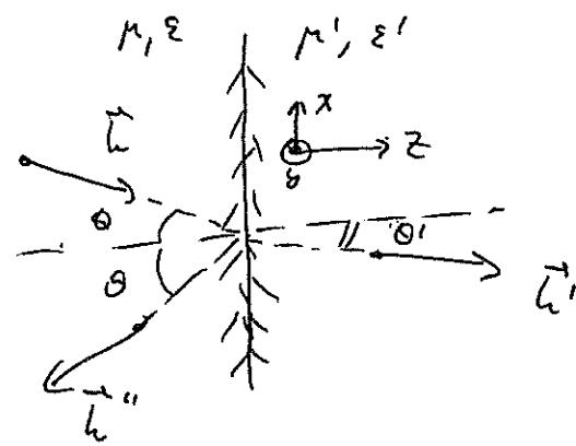
$E_0'' = 0$  for polarization  $\parallel$  to the plane of incidence
