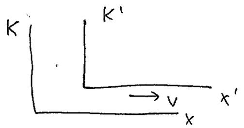
$$\Lambda^{\mu}_{\nu} = \begin{pmatrix} \gamma & -\beta\gamma & 0 & 0 \\ -\beta\gamma & \gamma & 0 & 0 \\ 0 & 0 & 1 & 0 \\ 0 & 0 & 0 & 1 \end{pmatrix} \text{ for a boost along the } x\text{-axis}$$
