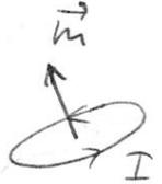
• loop of current carries magnetic dipole  $\vec{m}$
