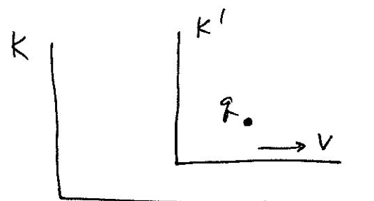
$$\begin{pmatrix} E_x \\ E_y \\ E_z \end{pmatrix} = \frac{q \gamma}{[\gamma^2(x-vt)^2 + y^2 + z^2]^{3/2}} \begin{pmatrix} x-vt \\ y \\ z \end{pmatrix}$$
