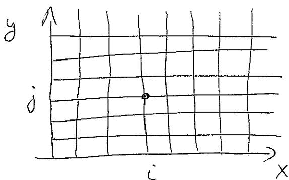
$$\nabla^2 \Phi = \frac{\partial^2 \Phi}{\partial x^2} + \frac{\partial^2 \Phi}{\partial y^2} = 0$$
