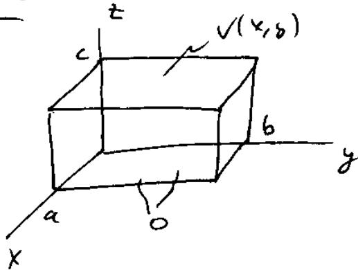
$$\Phi(x, y, z) = \sum_{n, m=1}^{\infty} A_{nm} \sin\left(\frac{\pi n}{a} x\right) \cdot \sin\left(\frac{\pi m}{b} y\right) \sinh\left(z \sqrt{\left(\frac{\pi n}{a}\right)^2 + \left(\frac{\pi m}{b}\right)^2}\right)$$
