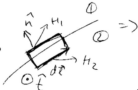
$(\vec{H}_1 - \vec{H}_2) \cdot d\vec{l} = \vec{K} \cdot \hat{t} dl$ , where  $\vec{K}$  = surface charge density (amps/m).
