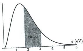
To locate the visible portion of the spectrum, note that the red end is at 700 nm which corresponds to a photon energy of  $\epsilon = hc/\lambda = 1.77$  eV, while the violet end is at 400 nm which corresponds to a photon energy of 3.1 eV. I've shaded this region in
