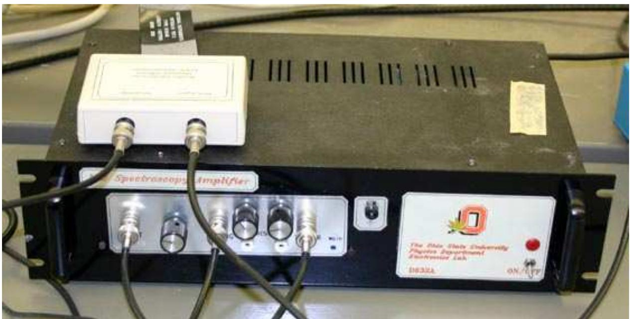
**Note:** The NaI Spectroscopy Amplifier and INTERFACE BOX were designed and built by the OSU physics department electronics shop. The spectroscopy amplifier is described in detail in a note titled D632A, which can be obtained from the electronics shop and is included in the special notes for P616 experiment N3.
