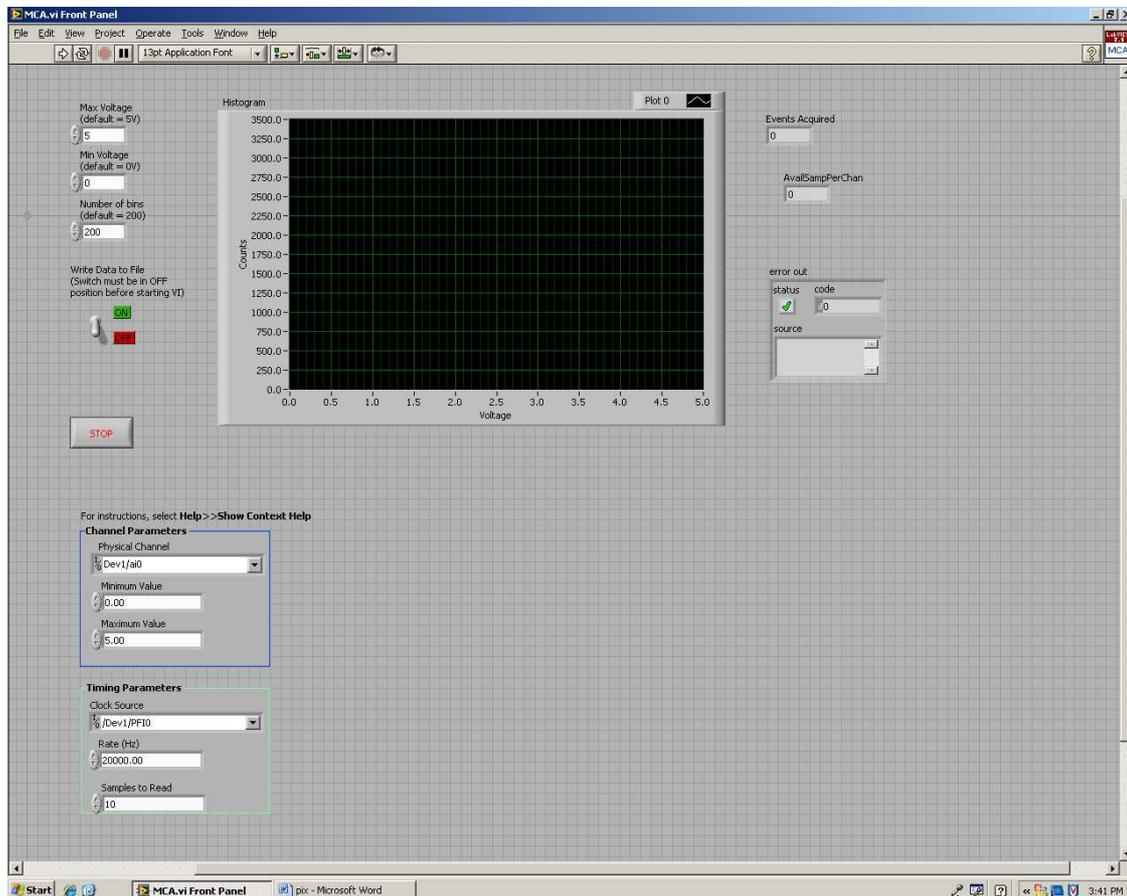
The above will display a histogram (once data collection has started) in which the vertical (y) axis gives the number of pulses (counts) in a bin (range) of voltages (x axis). As we collect data, the number of counts in a given bin will build up on the y axis.
