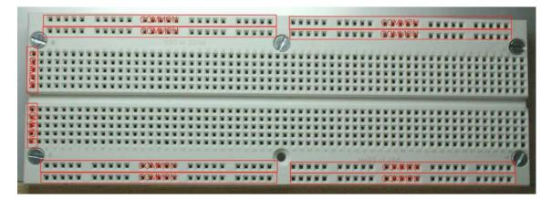
The connectivity is evident from the bottom side of the bread-board which shows stripes of metal that are isolated from each other.
