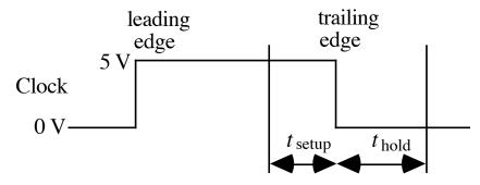
the data on J and K must be stable for at least  $t_{\text{setup}} + t_{\text{hold}}$ .
