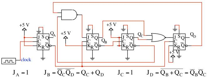
$J_{B} = \overline{\overline{Q}_{C}}\overline{\overline{Q}_{D}} = Q_{C} + Q_{D}$  $J_A = 1$
