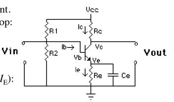
DC voltage gain (G) for a common emitter amp:
