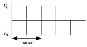
Plot the output voltage for RC = T/20, T/2, T/2, T/2, where T = period, for both circuits (6 plots in all). Of the six cases which output is most like integration, and which is most like differentiation of the input signal?
