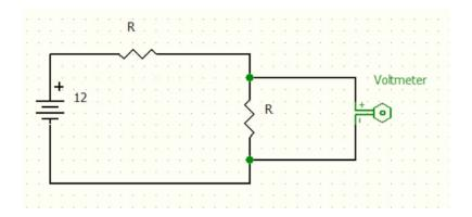
**8.** Find the current going through each resistor and the voltage drop across each resistor. The resistor values are in Ohms.
