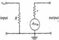
4. Calculate the DC and AC voltage gain of the amplifier (Simpson P255, problem 27). Assume  $R_L = 1$  M $\Omega$ ,  $h_{ie} = 2 K\Omega$ ,  $h_{re} = 10^{-4}$ ,  $h_{fe} = 100$ ,  $h_{oe} = 10^{-5} \ mhos$ . Note:  $R_L$  is not shown in the figure.
