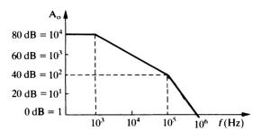
2. Simpson: problem 18, page 410. Although the output resistance of most op amps is extremely low when negative feedback is used, a typical inexpensive op amp can supply only a maximum current of approximately 25 mA. Calculate the maximum amplitude sinusoidal input (at low frequencies ~ 1 kHz) that will produce a non-distorted output across  $R_L = 100 \Omega$ . Repeat it for  $R_L = 1 k\Omega$ .
