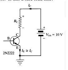
5. Simpson P252, problem 11. Calculate  $I_C$  and  $V_{CE}$ . The transistor is silicon and has a  $\beta$  of 100.
