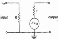
4. Calculate the DC and AC voltage gain of the amplifier (Simpson P255, problem 27). Assume  $R_{\rm L}=1$  M $\Omega$ ,  $h_{ie}=2~K\Omega$ ,  $h_{re}=10^{-4}$ ,  $h_{fe}=100$ ,  $h_{oe}=10^{-5}~mhos$ . Note:  $R_{\rm L}$  is not shown in the figure.
