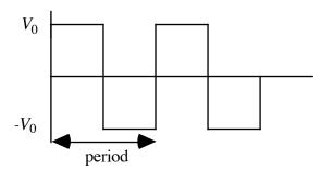
Plot the output voltage for RC = T/20, T/2, 20T, where T = period, for both circuits (6 plots in all). Of the six cases which output is most like integration, and which is most like differentiation of the input signal?
