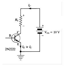
Note: The transistor is an NPN. How is  $I_C$  related to  $I_E$ ? Use Kirchhoffs's law to determine  $V_{CE}$ .
