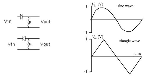
Note: The output is measured across the resistor after the input voltage has passed through the forward biased diode. In (b), how does the battery power affect the input signal?
