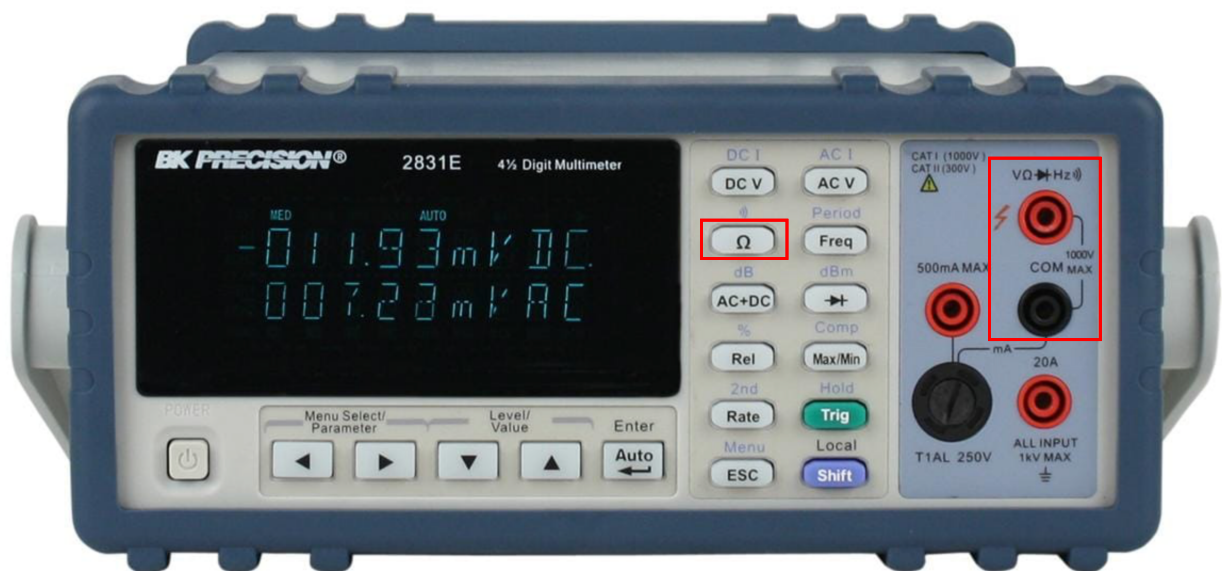
Fig. 1: BK Precision 2831E multimeter. The connector on one end of a banana cable should be inserted into the two connectors inside the red box on the upper right-hand corner. Push the white button labelled “ \Omega ” inside the red box to set the multimeter to measure resistance.
