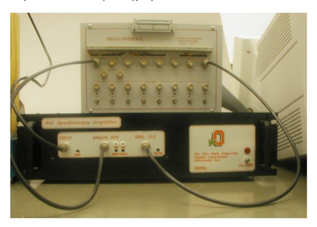
**Note:** The NaI Spectroscopy Amplifier and MAC/LC INTERFACE were designed and built by the OSU physics department electronics shop. The spectroscopy amplifier is described in detail
