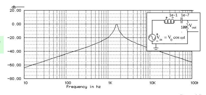
Bode plot of magnitude of  $V_R/V_{in}$  vs. frequency
