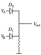
$$V_{\text{out}} = V_{\text{A}} \text{ or } V_{\text{B}} \text{ if either diodes conduct}$$
