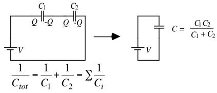
*Total* capacitance is *less* than individual capacitance!
