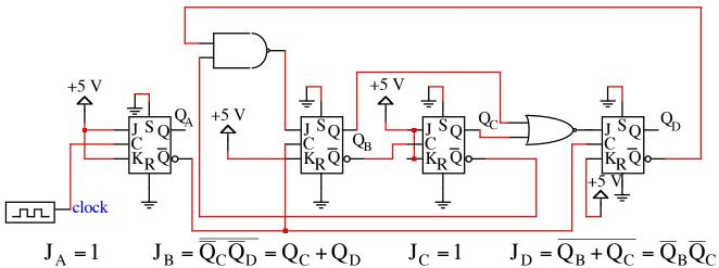
$J_B = \overline{\overline{Q}_C \overline{Q}_D} = Q_C + Q_D$  $J_A = 1$
