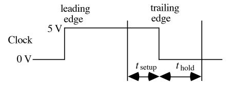
the data on J and K must be stable for at least  $t_{\text{setup}} + t_{\text{hold}}$ .
