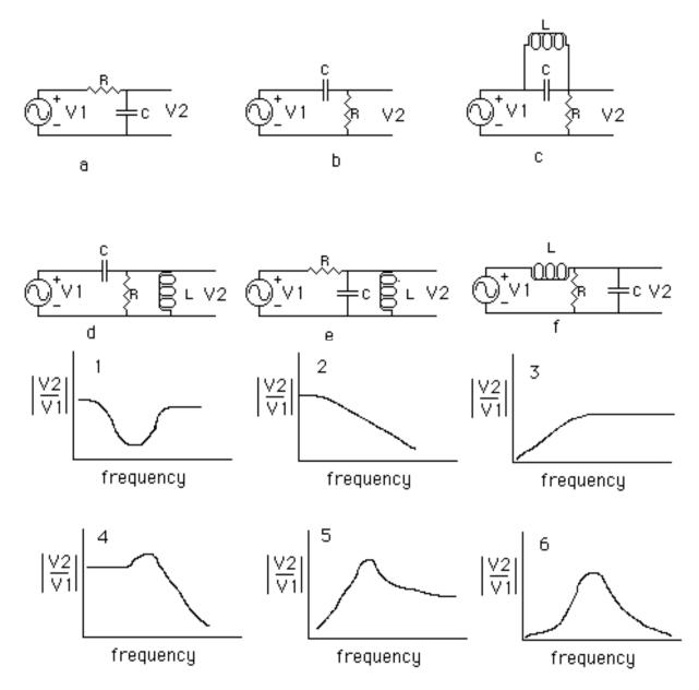
6. For each of the six circuits in problem 5), find an expression for the gain  $|V_2/V_1|$  in terms of *R*, *L*, and *C*.
