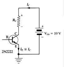
5. Calculate  $I_C$  and  $V_{CE}$ . The transistor is silicon and has a  $\beta$  of 100.
