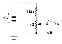
**4.** Calculate the voltage between A and B. What is the polarity of  $V_{AB}$ ?
