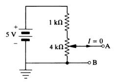
**4.** Calculate the voltage between A and B. What is the polarity of  $V_{AB}$ ?
