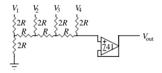
The output voltage for this circuit is:
