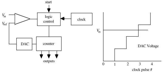
When  $V_{\text{DAC}} > V_{\text{in}}$  the logic circuit stops the clock and the counter outputs a binary number which is just the number of clock pulses.
