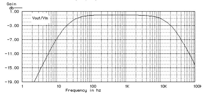
Let's design an audio filter using low and high pass RC circuits.
