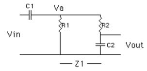
Working from right to left, we have:  $V_{out} = V_a X_2 / (X_2 + R_2)$
