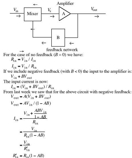
For this example the input impedance with negative feedback is *much larger* than the no feedback case.
