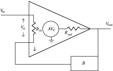
The above figure is a model of the op amp with negative feedback. Assume that  $V_{in}$  is grounded, and we put a voltage V at the output of the amp. The feedback network puts  $BV_{out}$  (B < 0 for negative feedback) back to the input. This voltage appears across the input impedance as  $V_{d}$ .
