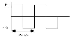
Plot the output voltage for RC = T/20, T/2, 20T, where T = period, for both circuits (6 plots in all). Of the six cases which output is most like integration, and which is most like differentiation of the input signal?
